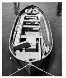
Showing clear space in boat with equipment stowed in compartments.
