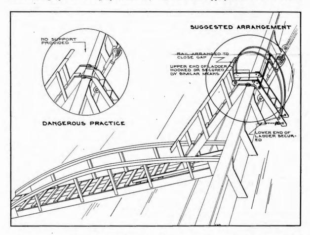
leaving an unprotected space between the ship's rail and the end of the handrail on the ladder. Probably all three lives might have been saved had an adequate guard rail been installed at this danger point.
