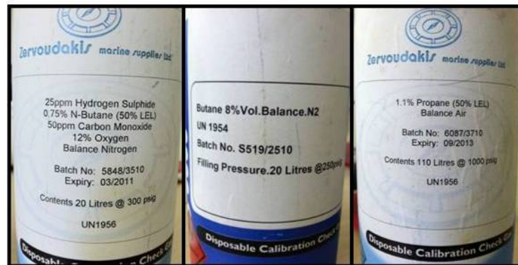
Figure 5-9 Example span gas: 4 gas; 8% butane, balance nitrogen (N 2 ); and 50% LEL
