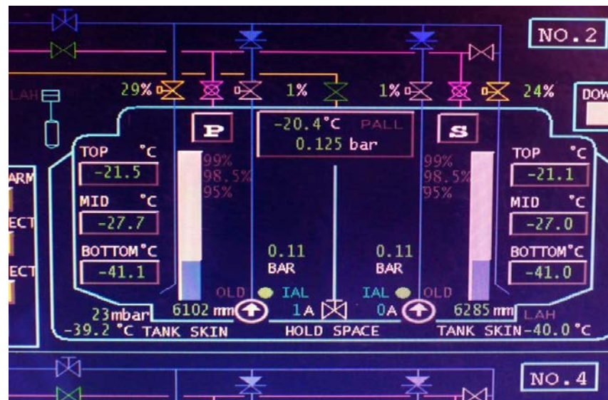
Figure 5-14 Temperature indicating device readings on an LPG gas carrier
