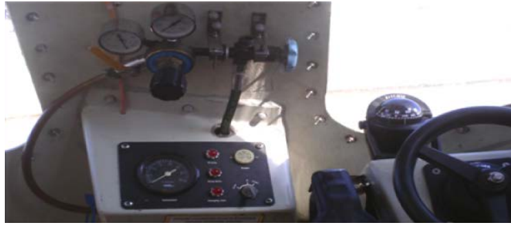
Figure 10-1 Self-contained air support system
