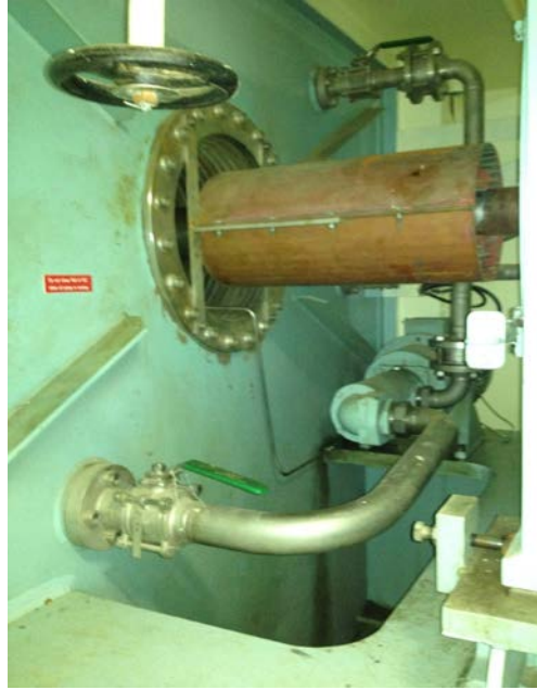
Figure 8-20 Lubricated bulkhead shaft seal passing through the gas tight bulkhead on an LNG gas carrier
