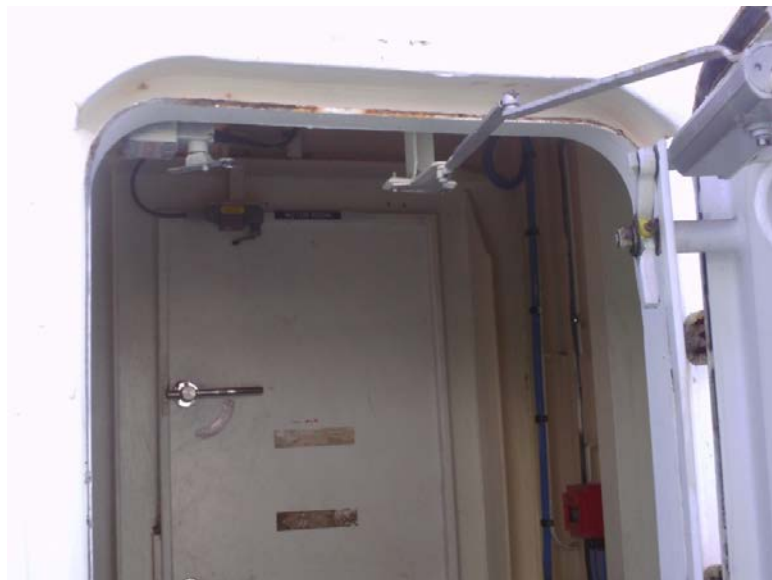
Figure 7-2 Self closing mechanism, door open, and door closed indicator
