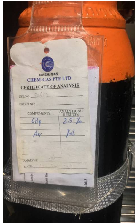
Figure 5-3 LNG gas carrier cycled gas detection span gas analysis certificate
