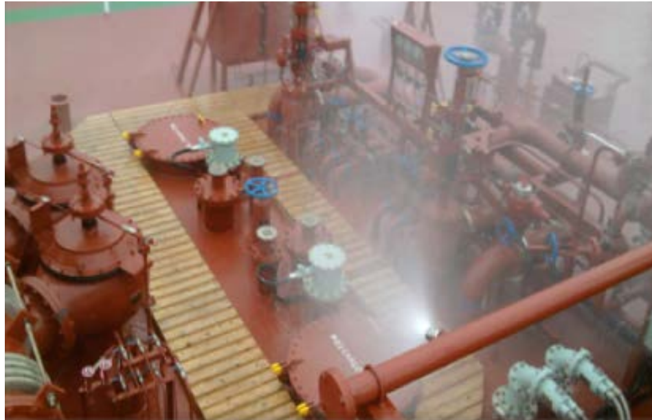
Figure 14-2 Deck water spray system (tank domes)
