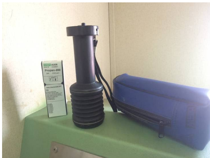
Figure 5-13 Portable gas meter
