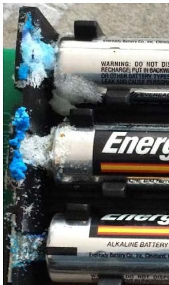
**Figure 1: General Leakage Example
