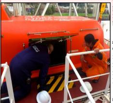
the vessel and company were not following shipboard and SMS procedures for the upkeep of critical lifesaving equipment, including the maintenance of lifeboat engines and expired SART batteries.
