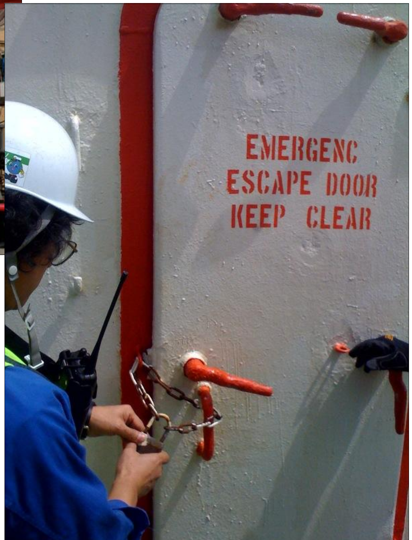
Top: Port State Control team is challenged by gangway watch, upon arrival at vessel (USCG Sector Anchorage) Right: Improperly secured and labeled escape door, (USCG Sector Puget Sound).
